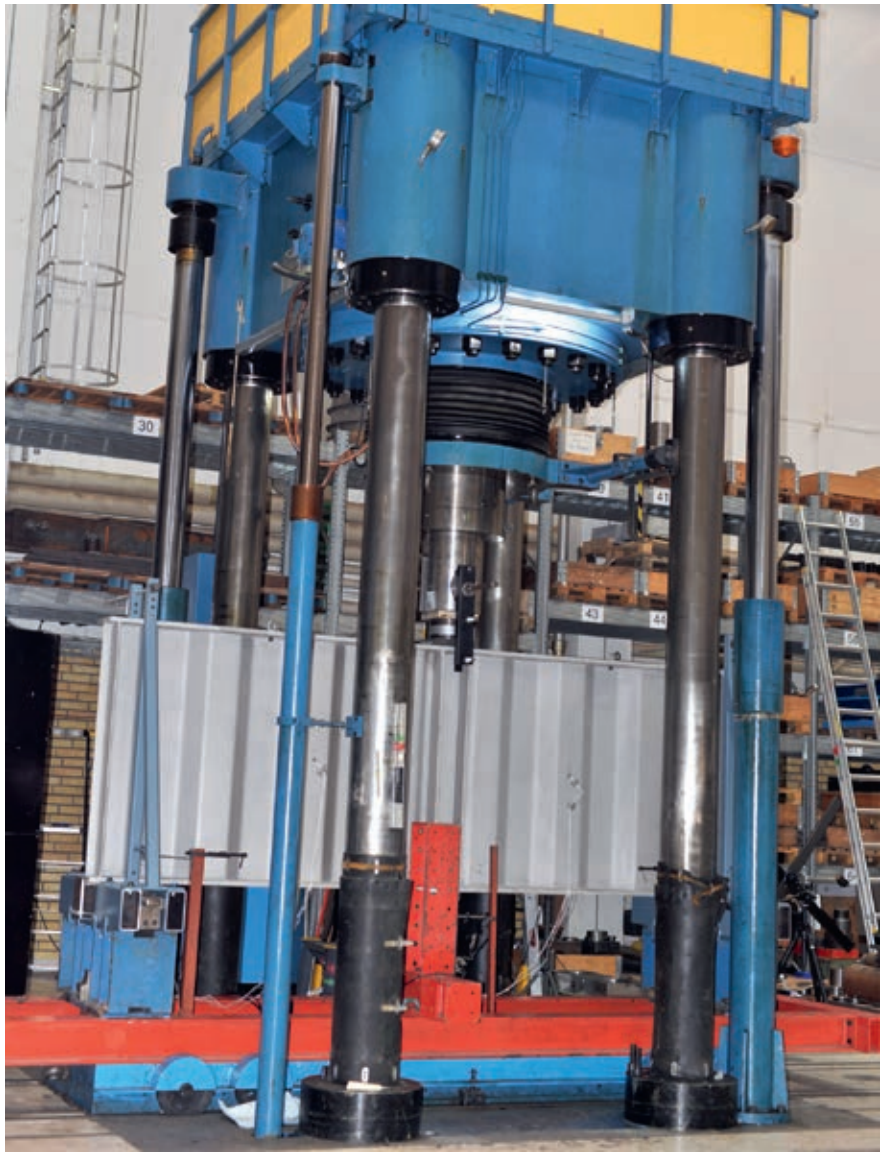
Fig. 5: Three-point bending test set-up
