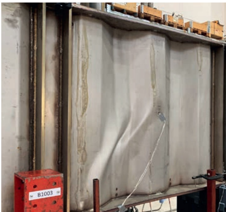
Fig. 7: ultimate deformation of the four tested girders; 1003–1004.
