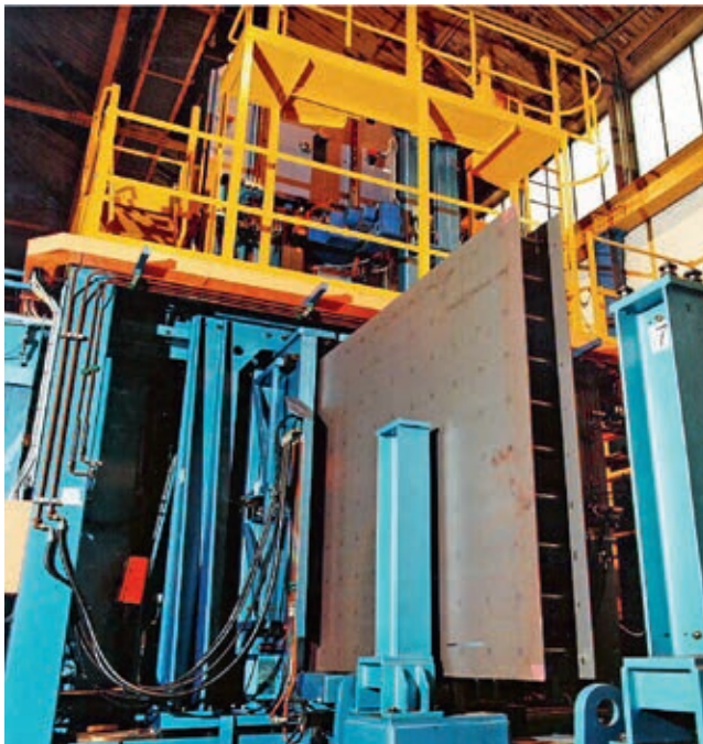
Fig. 4. A Friction-stir welding tool (left) to fabricate a bi-steel panel and a completed fabricated panel (under).
