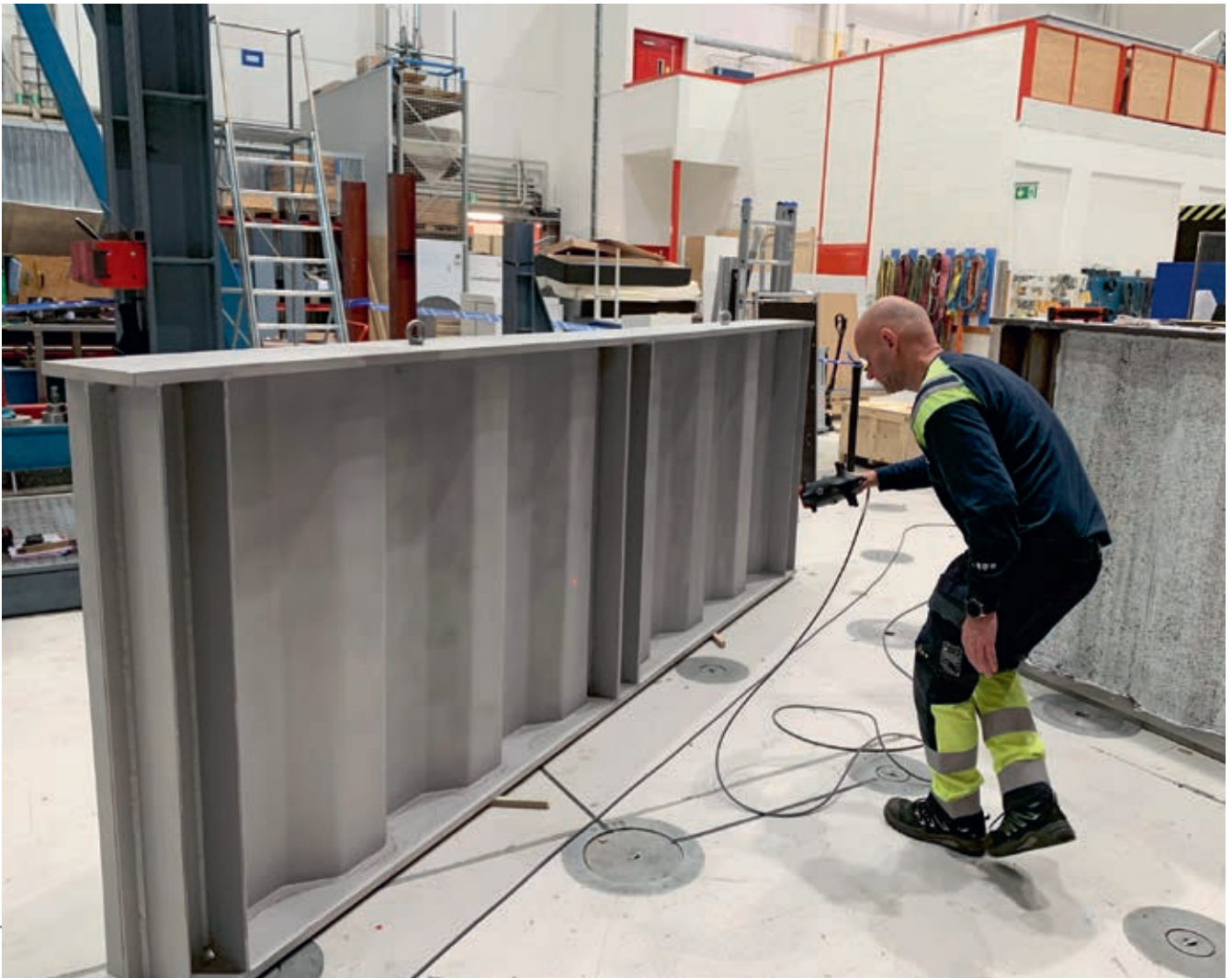
Fig. 1: A corrugated web stainless steel girders produced for the SUNLIGHT testing program during 3D laser scanning. Girder is 1.45 m deep with a web of 4- or 6-mm thickness
